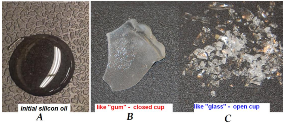
Fig. 15. Oil consistency transformation in an experiment: from (a) initially liquid then (b) to like a gum and (c) finally glass conditions takes near 2.5 days in high-temperature soaking.
